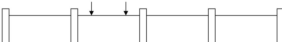
The subset of our field elements which are valid codewords are the fenceposts. Two other invalid codewords are noted by arrows. Errors occur during communication change the codewords, moving them along the fence line. To maximize our chances of guessing the correct codeword in spite of
