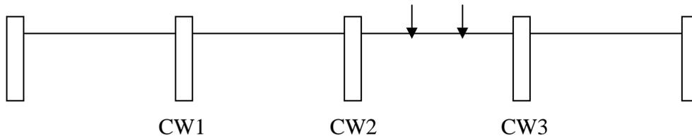
Looking at the diagram above, assume that codeword two has been transmitted. If one error occurs, it takes us one bit closer to codeword three, but we can see from the diagram that the obvious selection of the corrected codeword is still codeword two. If two errors occur, then the received codeword is closer now to codeword three than codeword two, and the decoder will select codeword three as the right one, which is a mistake.
